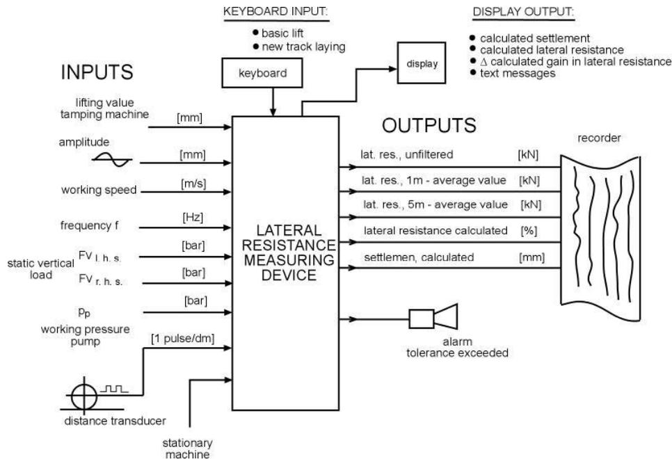
Figure 2: Composition of the dynamic, continuous RLD measuring device
