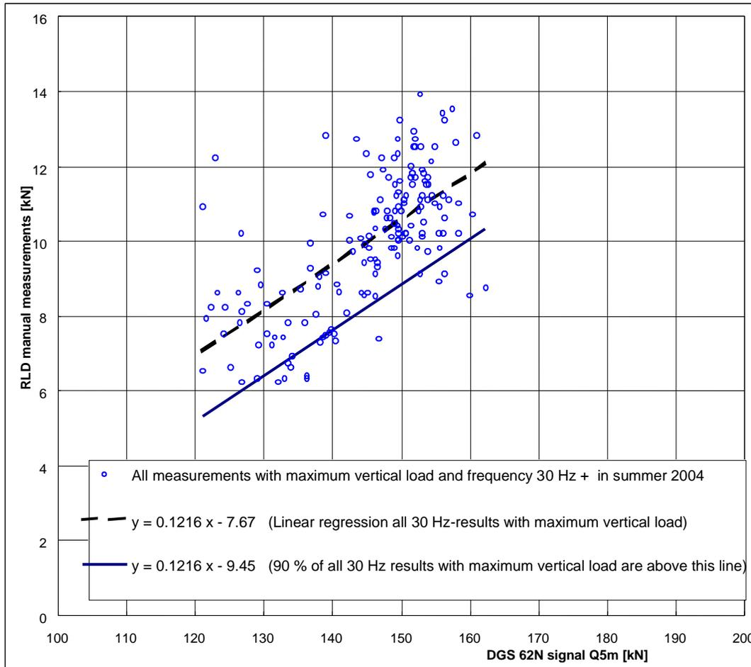
Figure 9: Correlation between manual measurements and DTS
