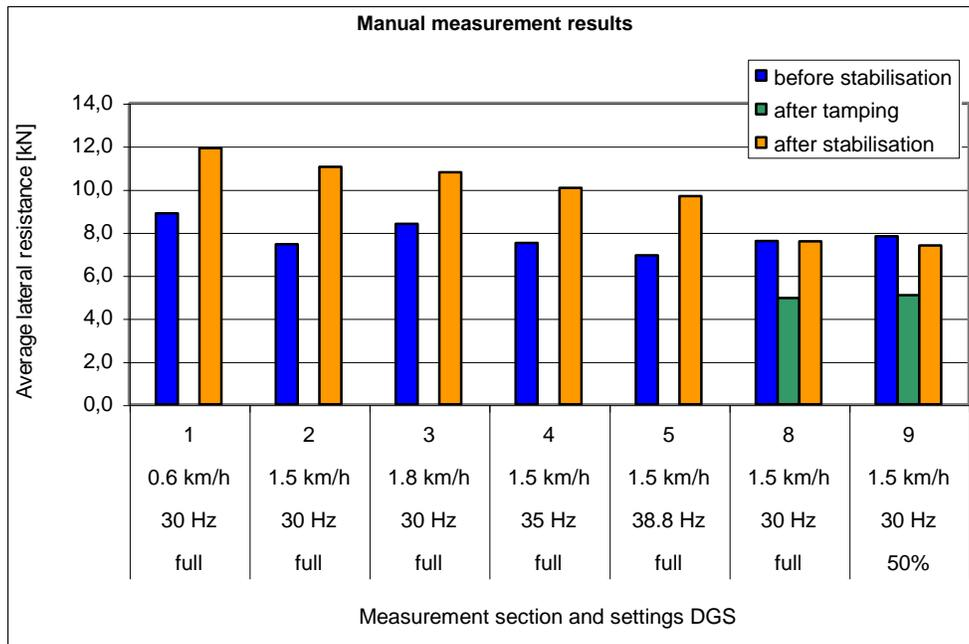
Figure 5: RLD values before and after tamping and following dynamic track stabilisation
