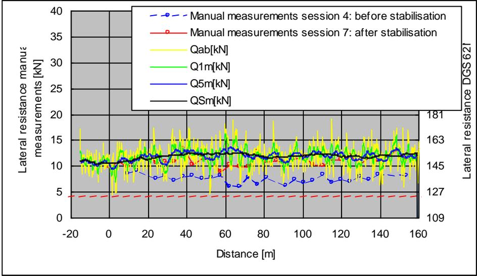
Figure 7: Comparison of RLD manual measurements and dynamic continuous measurement of RLD
