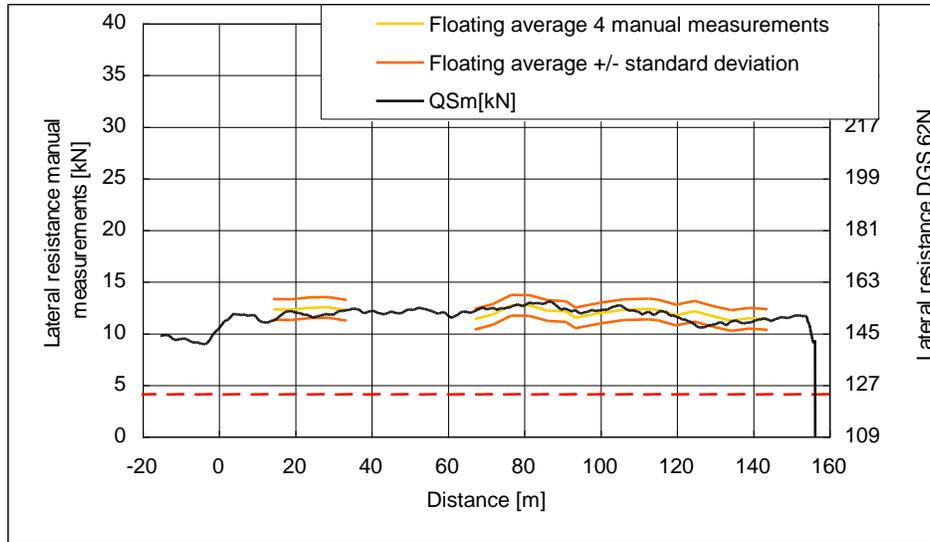
Figure 8: Comparison of average values of manual measurement and mechanical measurement
