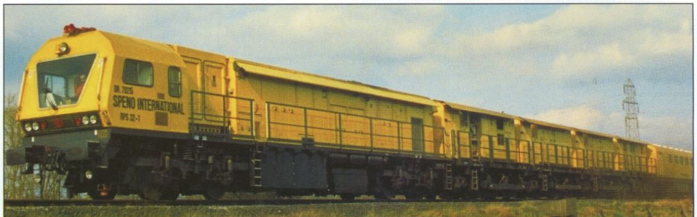
Fig. 1: Speno RPS 32 heavy-duty grinding train at work on Netherlands Railways
