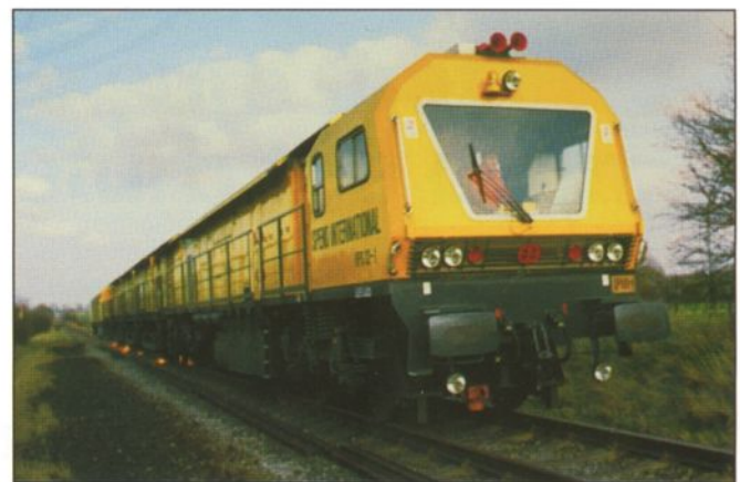
Fig. 4: The Speno RPS 32 heavy-duty grinding train was used during the pilot project to grind the plain track
